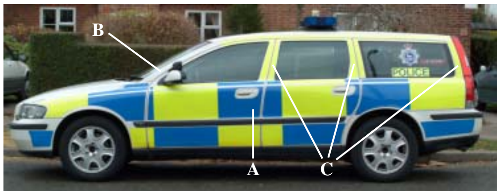
Photograph 4. Full battenburg side livery application
