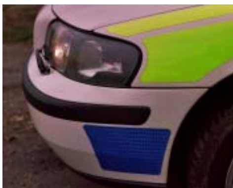
Photograph 5. Detail of front of full battenburg vehicle showing how livery film is 'cut around' headlamp and bumper
