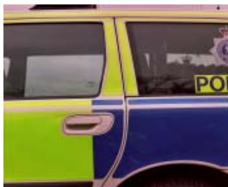
Photograph 6. Detail of centre of full battenburg vehicle showing how livery film is 'cut around' door handles and sharp curves on bodywork
